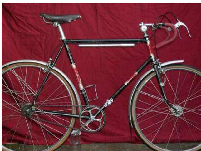
*David Palk's 1948 Paris Tour de France, built for 26" front and 27" rear wheels. You cannot fit it with equal size wheels - either 26 or 27, as one or other brake will not reach - and the top-tube takes on a horrible slope. it was, without doubt, built for odd wheels but rides very nicely he says!*
