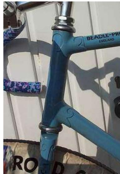
*Amazing cut-outs in the chainstays for fat tyres and chainset (left) and view of head lugs and fork crown on this unknown frame. It makes you wonder how much strength is left in the right stay and whether these cutouts were done by an amateur after the frame was built.*
