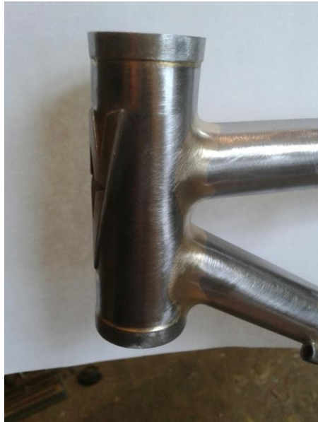
Brazing by Winston on a small custom-build frame with extended head tube
