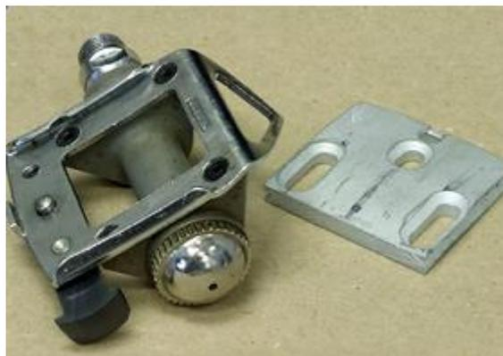
First generation (1970) M71 with chromed body, alloy shoeplate and square, rather than (later) round, window in pedal. Black lever is to release shoe with plate attached
