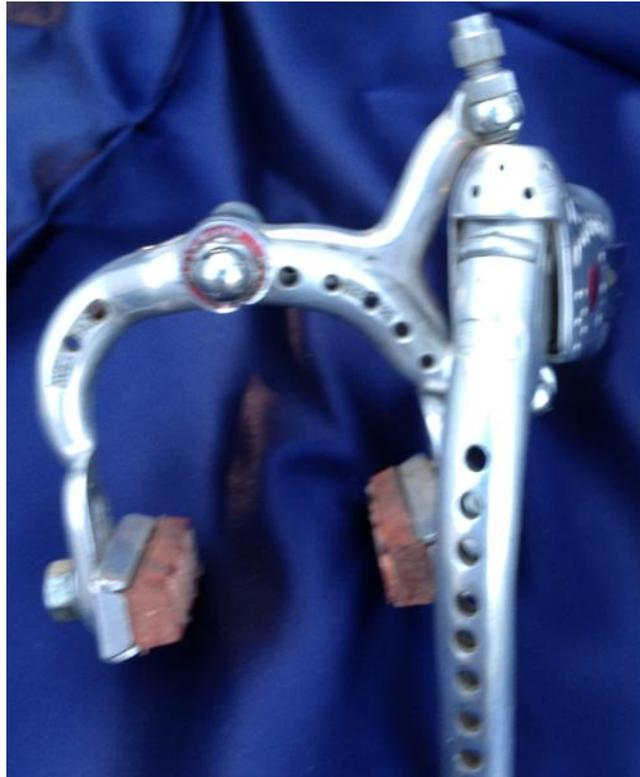
*Front view showing drilling on stirrup and lever
