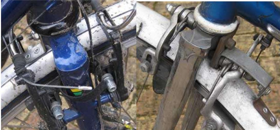
*Double V-brakes on the left and double side-pull on the right*
