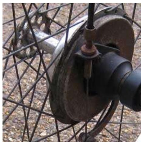
*Two views of a hub brake on rear axle of trike showing anchor point on right image*
